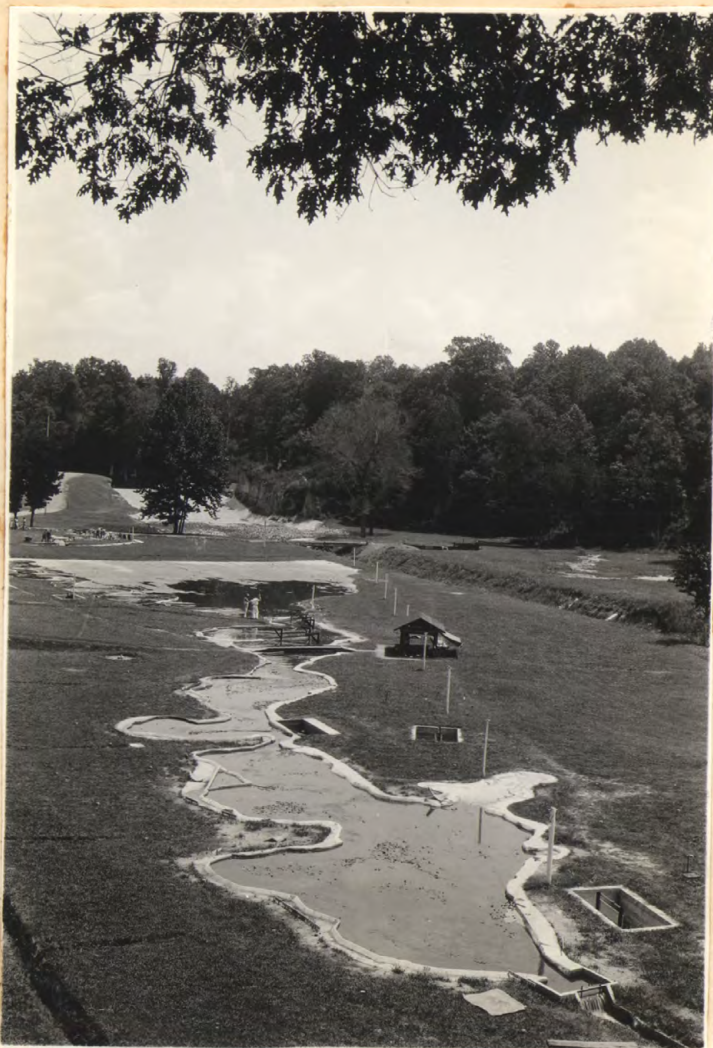
PLATE II GENERAL VIEW OF FIXED-BED, OUTDOOR MODEL, U. S. WATERWAYS EXPERIMENT STATION, VICKSBURG, MISSISSIPPI. HORIZONTAL SCALE 1 : 2400; VERTICAL SCALE 1 : 120. MODEL USED TO INVESTIGATE EFFECTS OF PROPOSED DREDGED CUT- OFFS BELOW LAKE LEE. UPPER LIMIT AT MILE 484, LOWER LIMIT AT MILE 762.7 .
